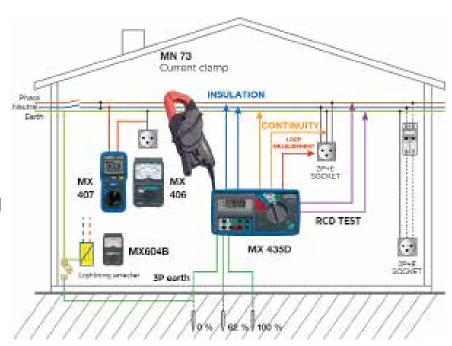
The purpose of electrical safety testing is to ensure the safety of people and property in the event of a fault on the installation. It can also be used for preventive maintenance, thus avoiding serious failures. To guarantee safety, the CENELEC HD 384 standard specifies the requirements applicable to electrical installations in buildings, with the following measurements in particular:
