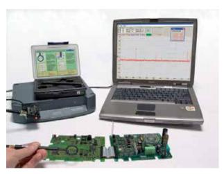
Measurements with the HX0083 proximity probe up to 10 cm from the target
