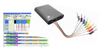
Self-contained bus-decoding probe powered via USB
