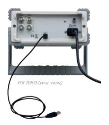
**SX-GENE v2.0** can be used to control a GX 1025 or GX 1050 arbitrary function generator, save and recall configurations and generate arbitrary signals.
