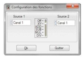
The Math functions: XY, differential, integral, curve smoothing Data export into EXCEL for processing in a spreadsheet
